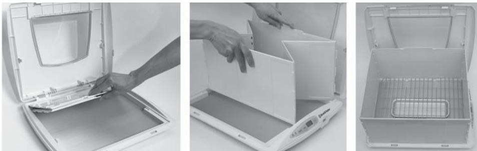
Place the water tray on the center of the heating plate. Place the wire rack into the enclosure with feet down. Lift the lid straight up from the rear hinges and place onto the top of the expanded box, fitting the guides on the lid into the matching grooves. Lower the lid to a closed position. Plug the power cord into the Proofer and then into an appropriate receptacle.
